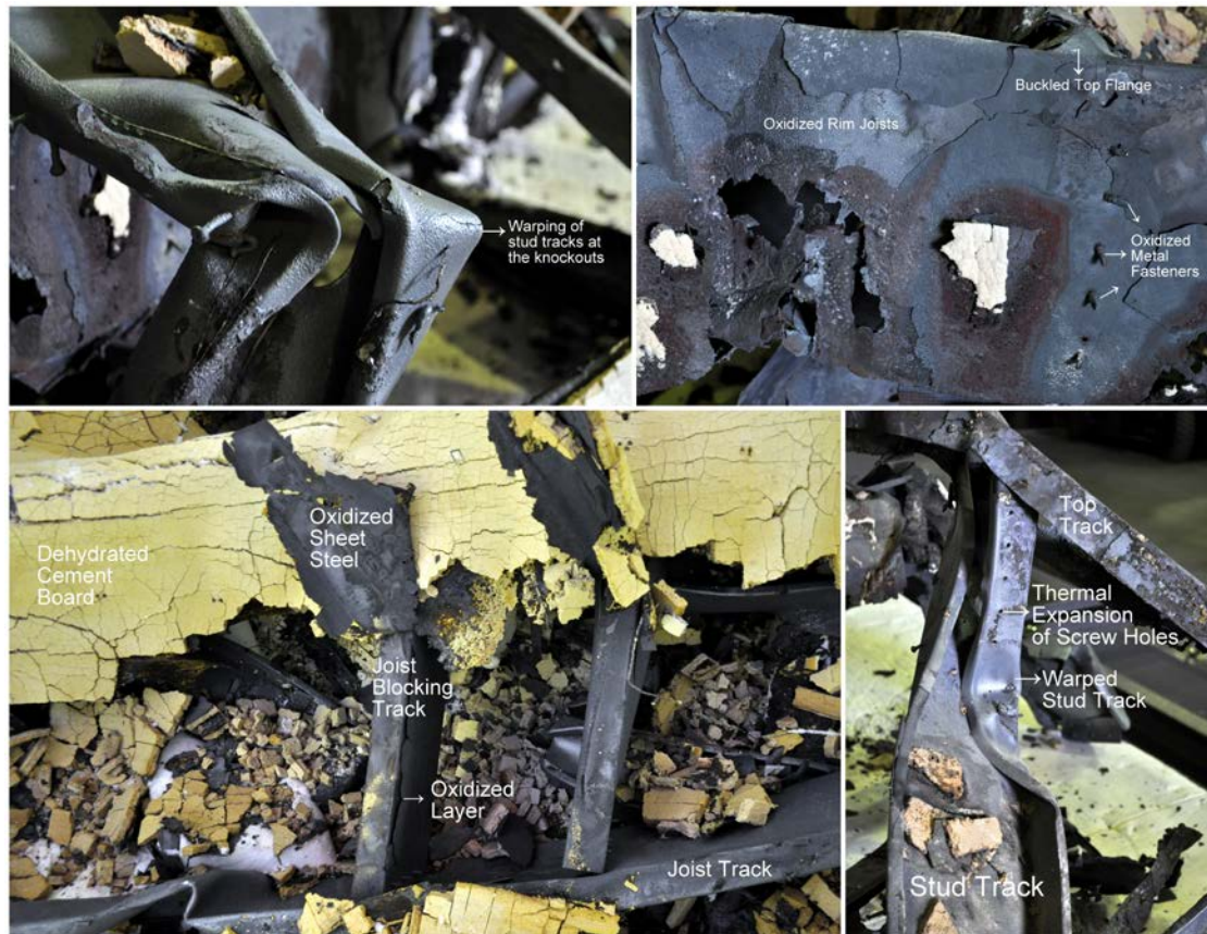
Figure 9. Failure patterns in the test specimen CFS01
