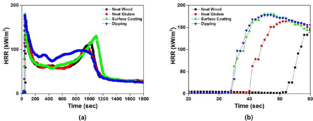
Figure 1. Cone calorimeter test with surface treated glulam
