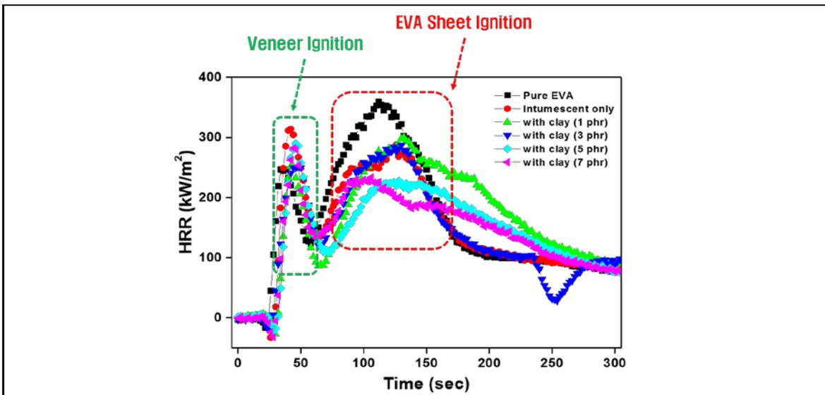
Figure 3. Cone calorimeter test with multi layered CLT
