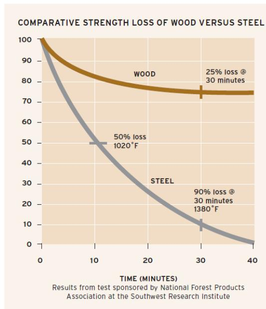
In order to take advantage of the laminated wood as a building interior material, analyzing the characteristics of the fire it is very important. Wood has very strong resistance to fire because wood form a carbide layer in the combustion process.
