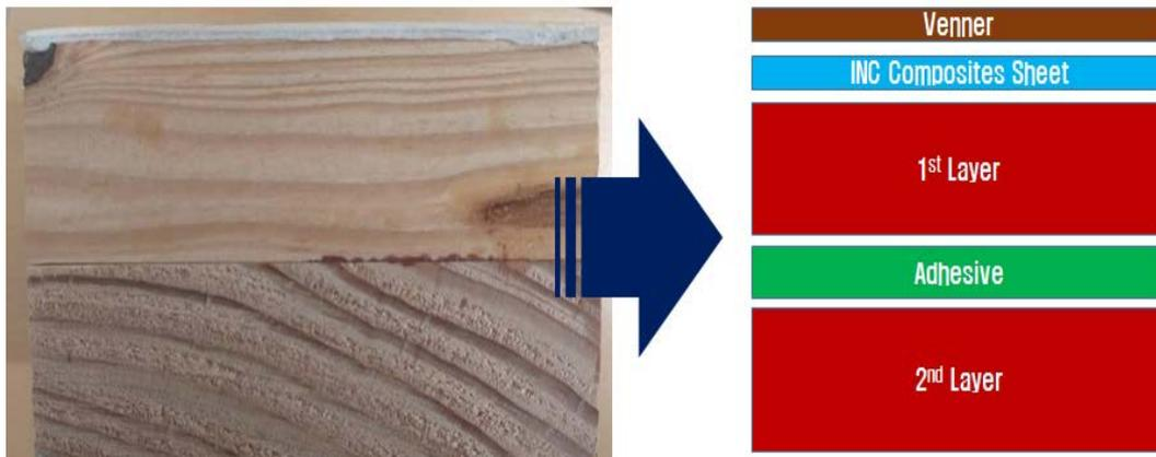
**Figure 2. The newly proposed multi-layered flame retardant CLT**
