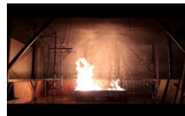
(B) 2 seconds after discharging air foam agent from JFEII approved heads
