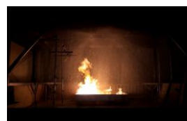
(B) Still burning 6 seconds after discharging air foam agent from JFEII approved heads
