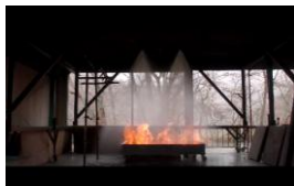
(A) 2 seconds after discharging air foam agent from test nozzles
