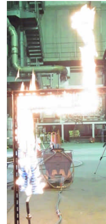
Photo 4 Free burning of the linear gas burner
