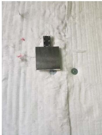
**Figure 1 Installation of plate thermometer on the façade and wall apart from facade**
