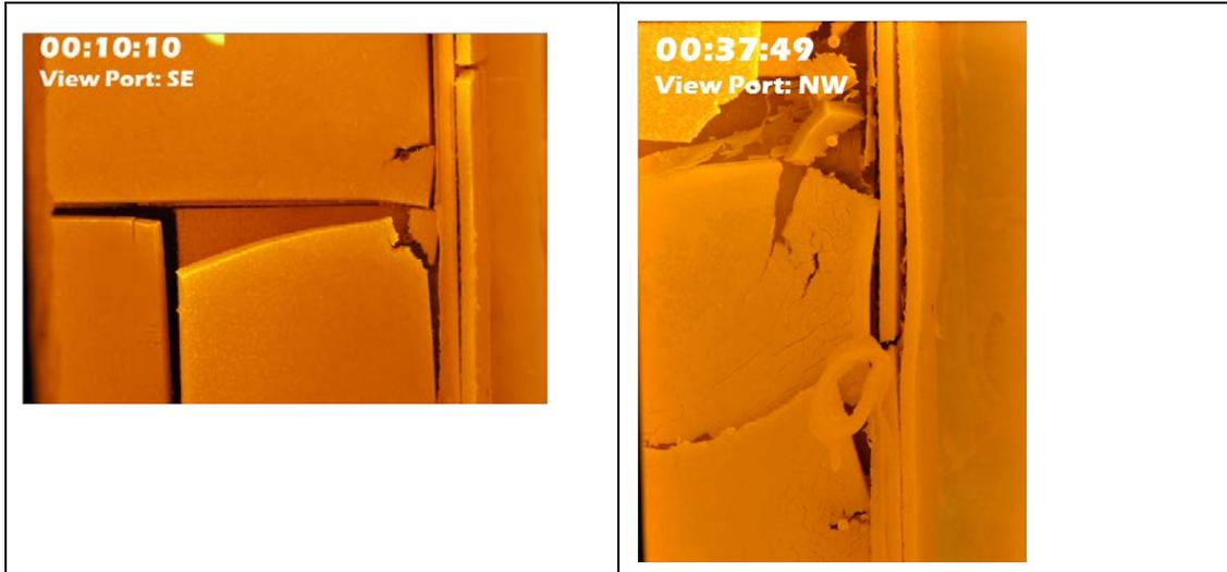
Figure below shows the collapsed roof panel and failure of the double stud connection.
