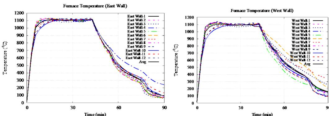
Results obtained by testing the cold-formed steel primarily consisted of temperature readings recorded by thermocouples instrumented at various locations of interest, as well as visual indication of failure modes and times to failure.
