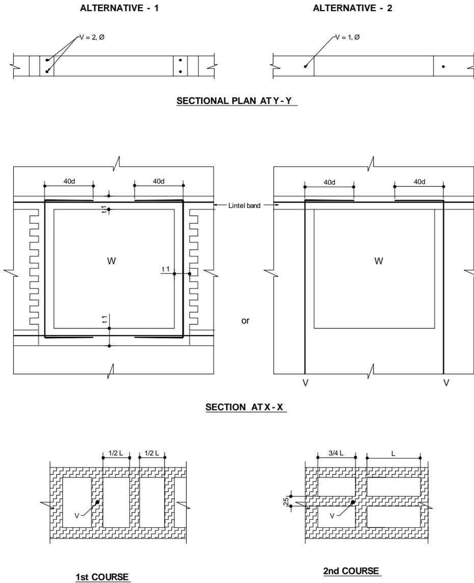
$\varnothing$  -- Diameter,                      W -- Window,                      V --- Vertical Reinforcing bar,
