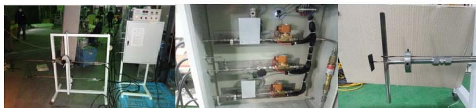
Figure 1 Burner system for bed mattress (entire photo : MFC photo : Burner head photo)
